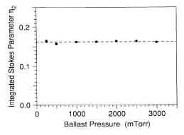
FIG. 6. Pressure dependence of  $\eta_2$  in neon at 25 eV electron energy. The dashed line represents the weighted mean of all data points, yielding a reduced- $\chi^2$  value of  $\chi_\nu = 1.45$  for six degrees of freedom. A ballast pressure of 1 Torr corresponds to a target density of roughly  $10^{10}$  cm<sup>-3</sup>.
