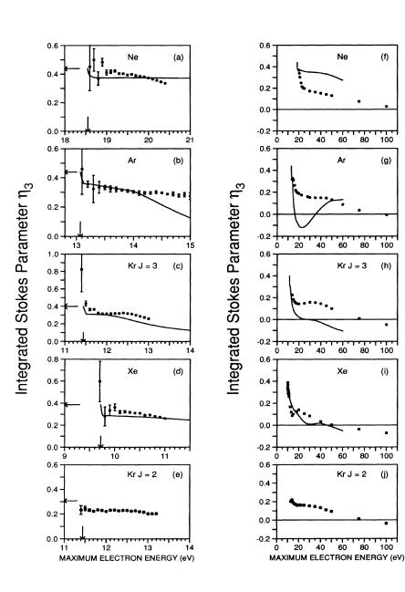
FIG. 9. Integrated Stokes parameter  $\eta_3$  as a function of maximum energy with the results of the DWB1 calculation indicated by the solid line. The kinematic-polarization limit and excitation threshold energy are indicated by arrows.
