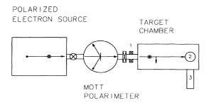
FIG. 3. Schematic diagram of the experimental apparatus showing the (1) spin rotator, (2) interaction region, and (3) optical polarimeter.
